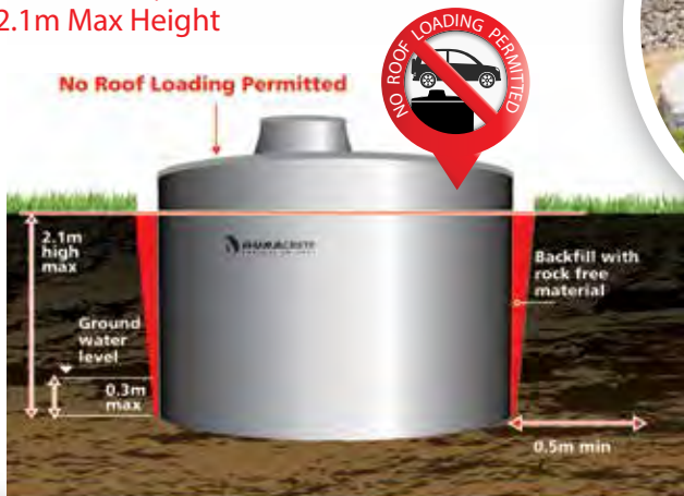
Standard 25,000L Tank Buried to 2.1m Max Height
